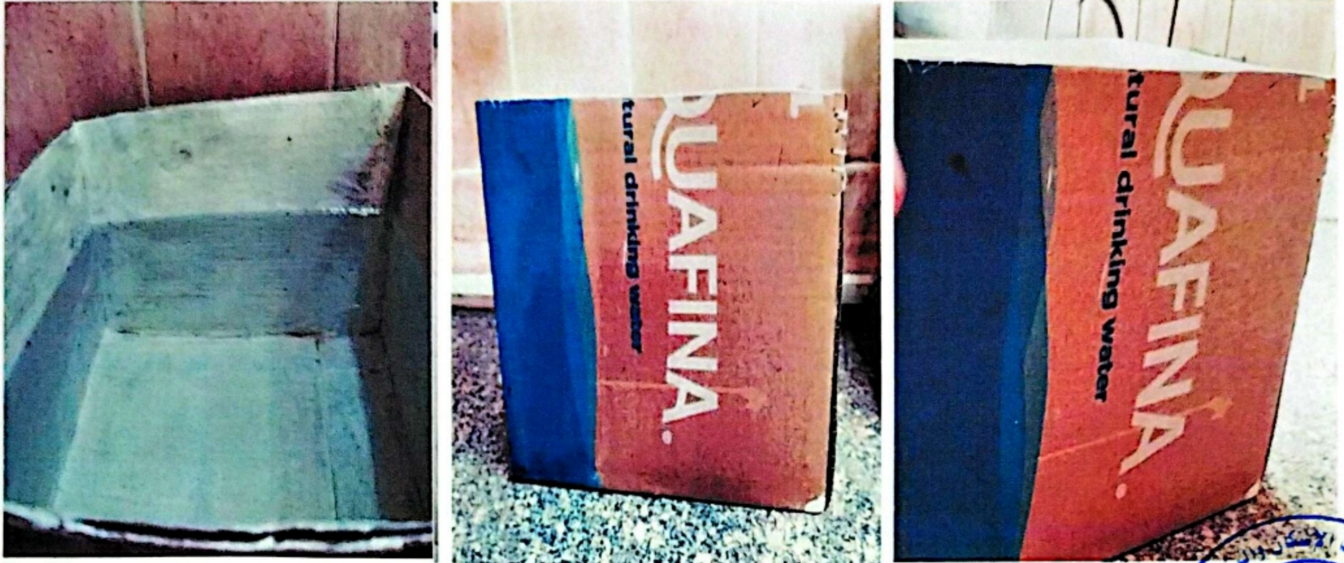
Fig (2) The water column level is 10cm for 10 days no water leakage appeared
