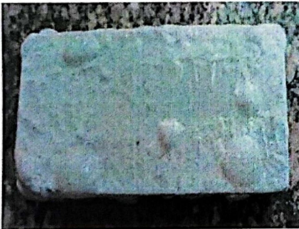
Fig 1: Sample after immersion in 5% HCl
