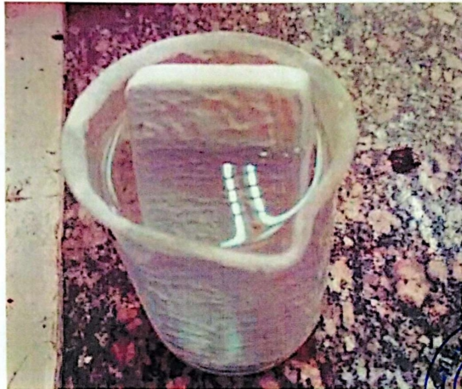
Fig 3: Sample after immersion in 15% Salt solution
