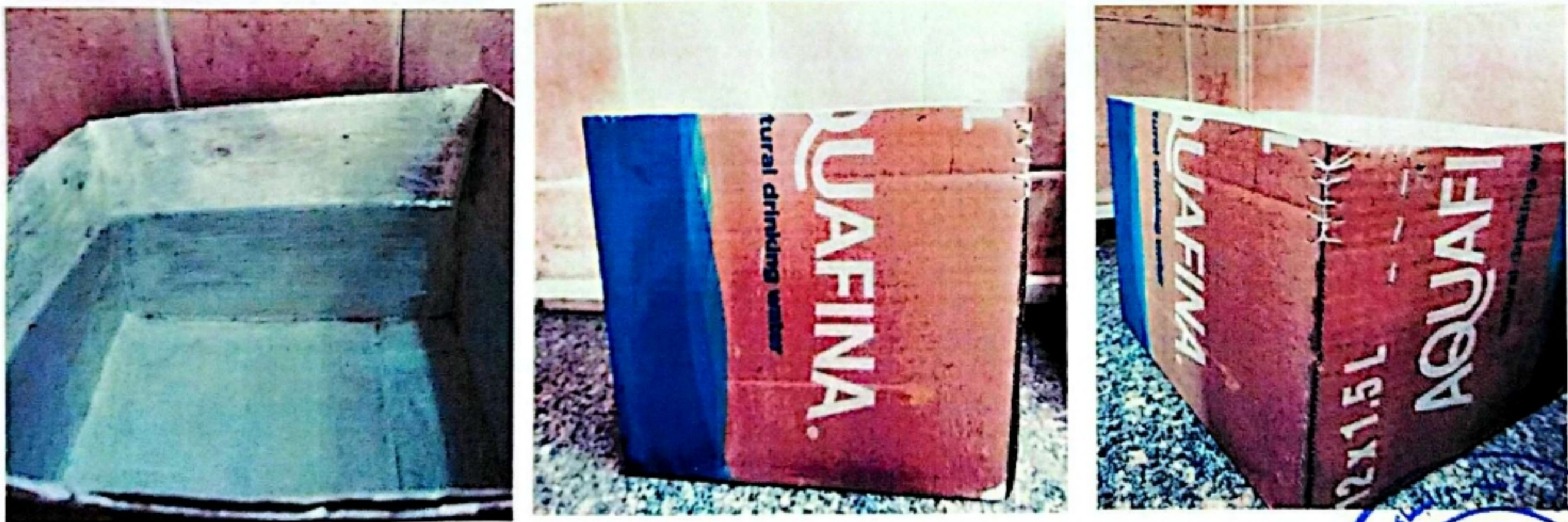
Fig (3) The water column level is 15cm for 15 days no water leakage appeared
