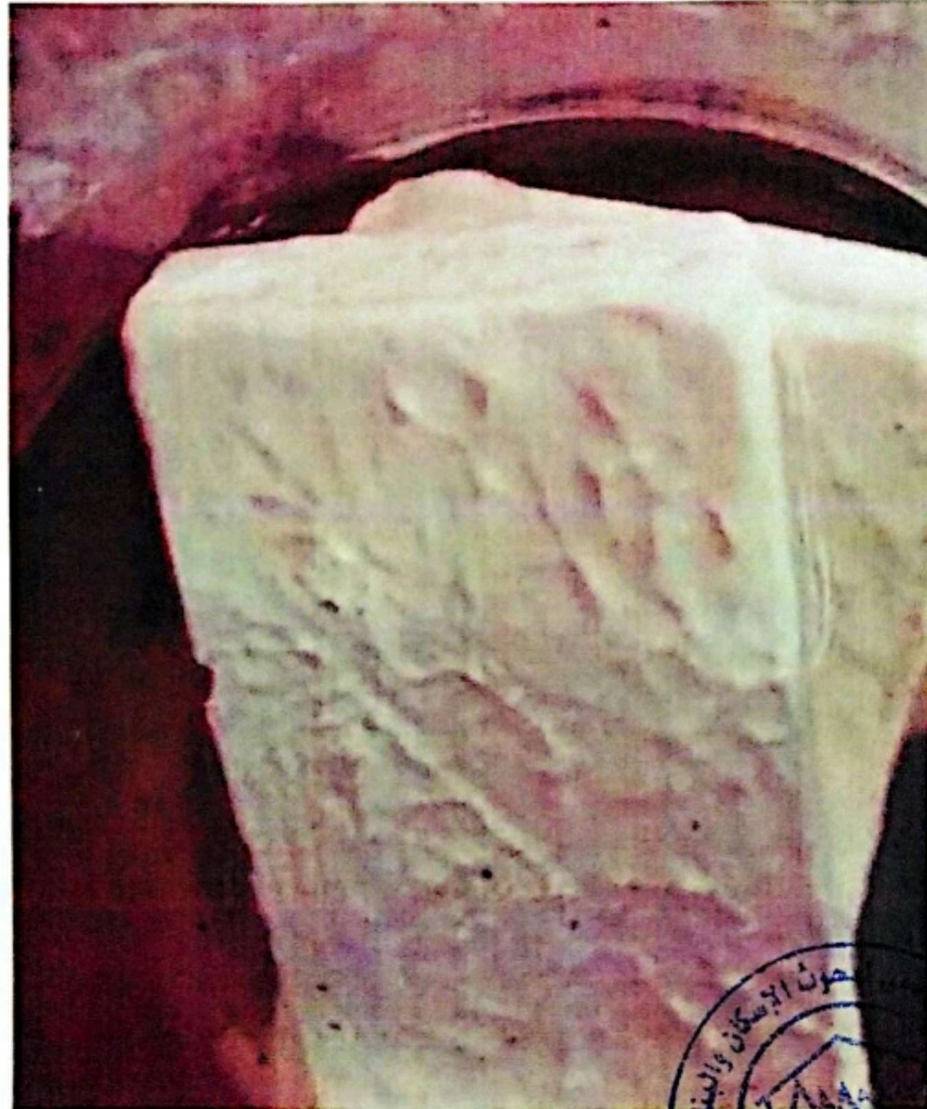
Fig 2: Sample after immersion in 5% Alkali solution
