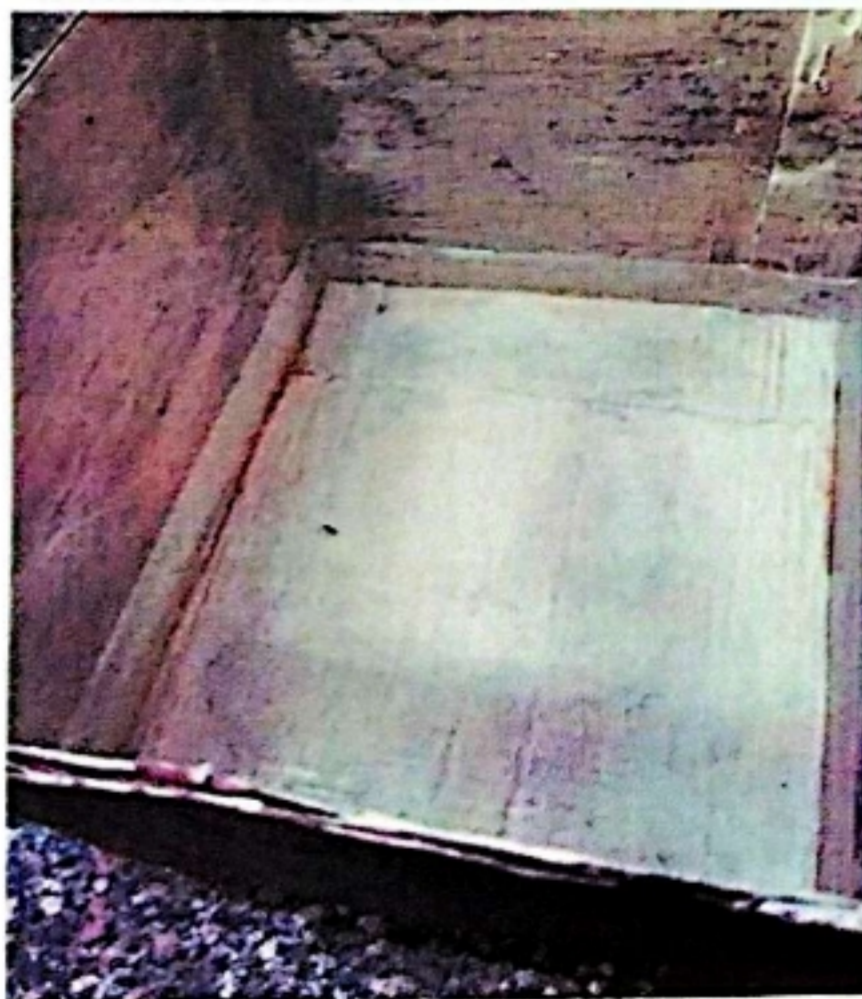
Fig (1) The water column level is 5cm for 10 days no water leakage appeared
